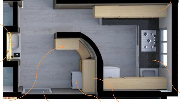
Overhead storage with 19mm thk MR ply finished with white laminate from inside and Rotal touche laminate – VW-1509 Vintage night teak from outside, with Dorma/Hettich fittings.
